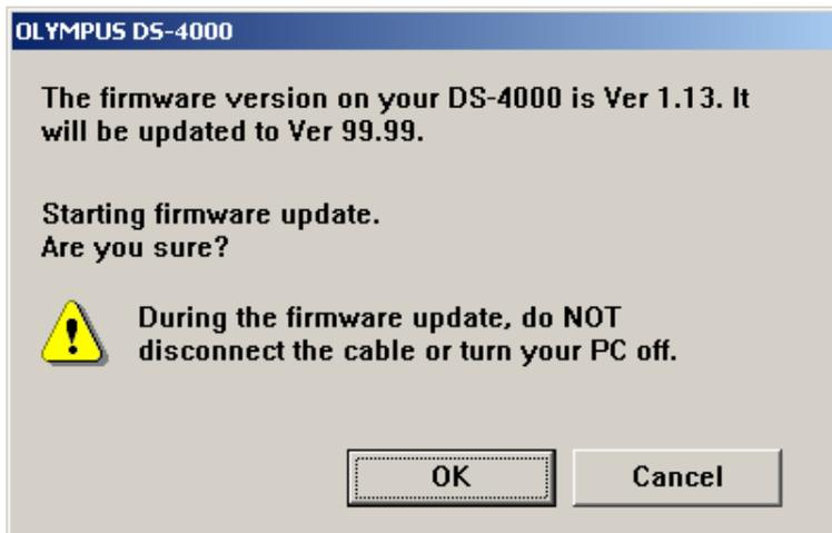
4. While the process of updating the firmware is taking place, the DS-4000 LCD will display “PROGRAM UPDATING...” DO NOT interrupt the process.
